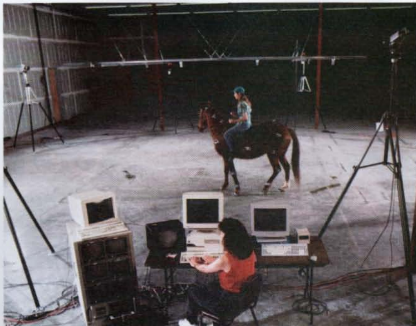
A typical optical set-up. First, highly reflective balls are attached to set points on the subject. Strobe lights then play over the capture area and sensors record the movement of the balls
